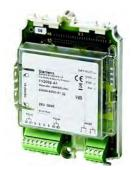
The module is a repeater in the FCnet/C-WEB. It is used for the extension of the range of the system bus. 1 repeater max. can be used between 2 stations. The distance between network module and repeater may be max. 1000 m.
