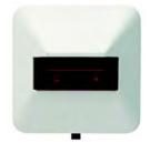
The Al322 alarm indicator is the visual parallel indication for fire detectors used on the SynoLINE300 detector line. It is provided with a dark red luminous element, fitted with LEDs. The alarm indicator is ideally used where the fire detector is difficult to see (e.g. hotel rooms, switching cabinets). The Al322 is suitable for surface wall mounting.
