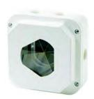
Retro-reflectors are characterized by the fact that an impinging light ray is reflected in parallel. The reflector does not need to be mounted at a right angle to the light ray. Vibrations and distortions in the wall where the reflector is mounted do not cause any disturbances either. Another advantage lies in the fact that possibly interfering light is also reflected in on itself and can thus not reach the receiver.
